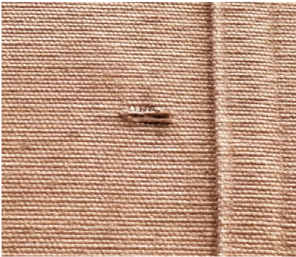
RIP IN FIRE CURTAIN
